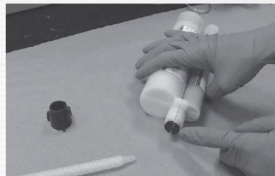
Figure 2 Remove any cap and plugs.
