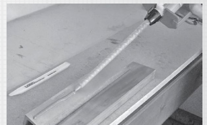
Figure 6 Position and dispense adhesive.
