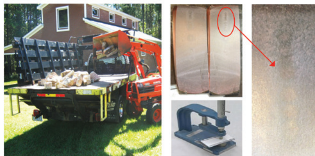
Figure 2. Impact resistance test. (2 mm thick aluminum substrate with 1 kg m Gardner impacts).
