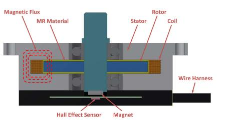
Torque feedback to the operator is generated through our proprietary "Direct Shear Mode" design, in which a rotor attached to a shaft shears magnetically responsive (MR) material against a fixed stator. As the current commanded by the vehicle steering controller to the TFD steering unit changes, a low-power (0-1 amp) coil generates a magnetic field that instantaneously changes the properties of the MR material and the subsequent torque feedback.
