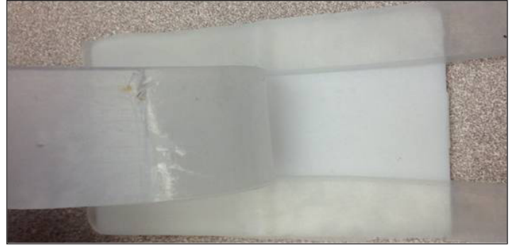
Figure 2: The photo above shows a TPE test specimen that has been overmolded with LSR before testing for peel strength. The strip shown is 25 mm wide.
