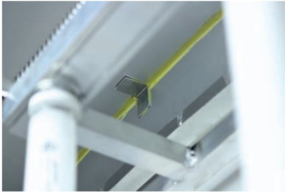
Figure 4 Adhesives can be used to bond joints in tight or difficult-to-reach areas.
