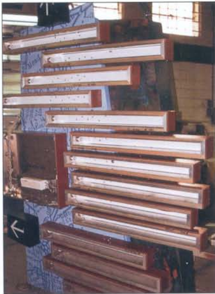
Tenant signs are backlit through routed out letters in the panels.
