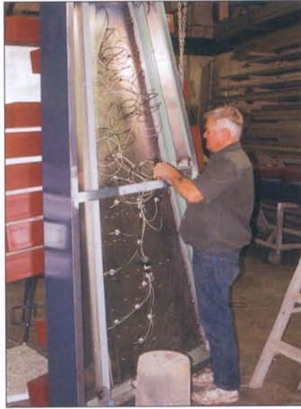
Tenant signs are backlit through routed out letters in the panels.
